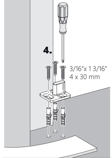
The fastening material must be provided by the customer and must be adapted to the local conditions!
